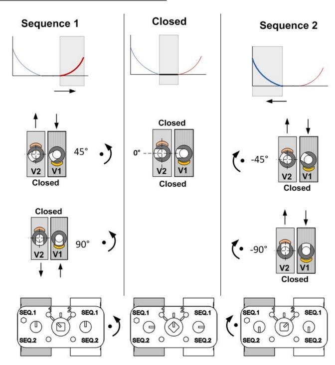
Both valves rotate in the same direction at the same time. Valve 1 (V1) has a disc oriented for CCW opening rotation. Valve 2 (V2) has a disc oriented for CW opening rotation. Each Cv has a Valve 1 and a Valve 2 version.
