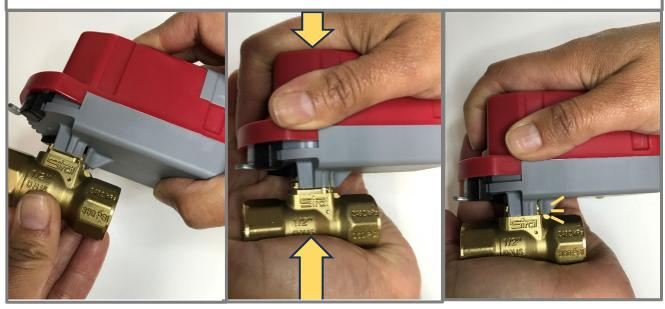
NOTE: Do not twist to disassemble. Pull hard and keep aligned.
