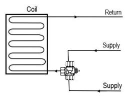
The Zone - series 3-way in switching applications, hot and cold supply water can be piped to either of the side ports and exit the bottom "AB" port for regulation by another 2-way valve; typically installed in the return pipe.
