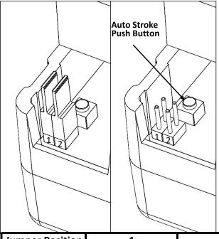
Direct/Reverse acting jumper is under wiring cover.
